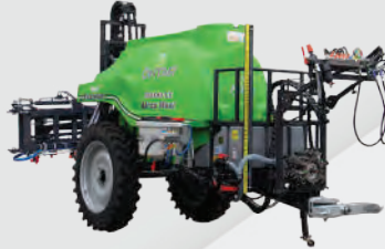
HIDRO RANGE : LIFTED WITH SELF LEVELLING HORIZONTAL HYDRAULIC BOOM
