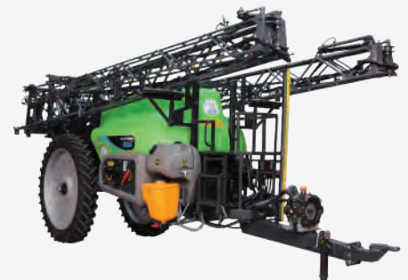
HIDRO L RANGE : PARALLELOGRAM HEIGHT ADJUSTMENT LATERAL FOLDING ADVANCED BOOM
