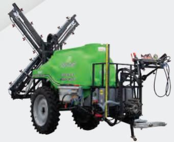
HIDRO X RANGE : LIFTED WITH SELF LEVELLING X TYPE HYDRAULIC BOOM
