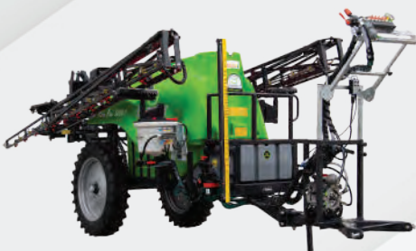
HIDRO L RANGE : PARALLELOGRAM HEIGHT ADJUSTMENT LATERAL FOLDING LIGHT BOOM
